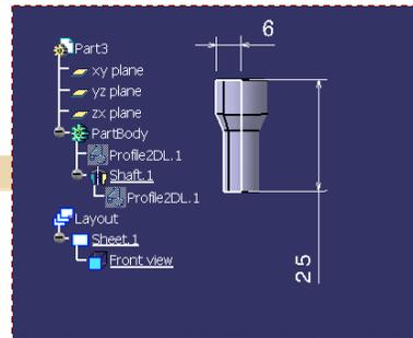
3 Create a new layout CATPart to design the air valve. Use the provided catalog to design the valve. Instantiate the 2D component, explode it, create the 3D profile and the shaft
