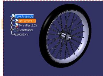
2 Change the tire and rim diameter from 32mm to 25mm
